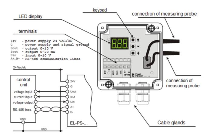
The device EL-PS-xxx does not use the input voltage Uin, however, the reading is available from the BACnet communication protocol and Modbus RTU.
