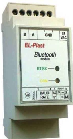
Bluetooth module facilitates wireless communication with visualization hardware including mobile phones, PDA, Notebook computers. The module ought to be connected to the controller using RS485 Master port. Communication parameters can be modified using appropriate jumpers located under a cover in the front panel of the module. The controller is equipped with a built-in antennae which facilitates communication in the radius of 100 m (Class 1). Module's operating manual is added to the module.
