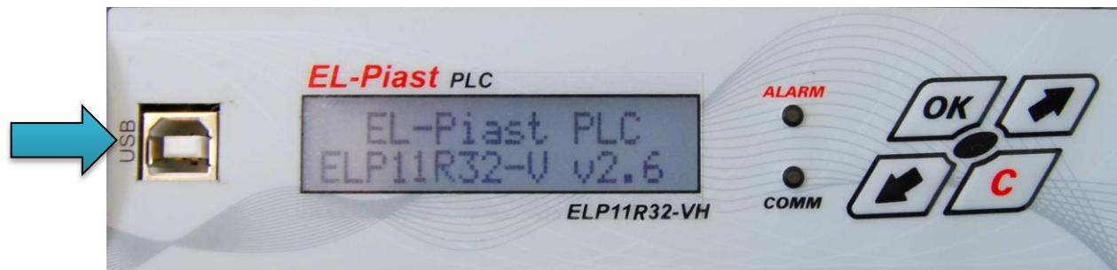
USB port is located on the upper controller panel. A standard USB cable is used to connect the controller with a PC. Appropriate drivers are stored on the CD attached to the controller or can be downloaded from EL-Piast Web site:
